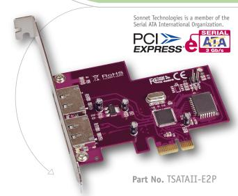
Are you planning to incorporate external data storage in your computer setup, but need a SATA host controller card to make the connection? Install a Tempo SATA E2P-it's an affordable solution for adding external SATA ports that enable you to hook up single and multi-bay SATA drive enclosures for your mass storage needs.
