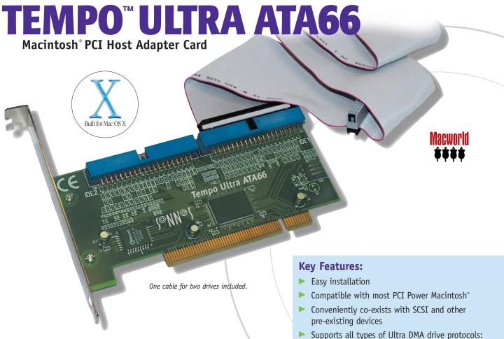
Why SCSI your Macintosh® when you can IDE it? With the Tempo Ultra ATA66 PCI Host Adapter from Sonnet Technologies you can now take advantage of the latest low-cost, high-capacity ATA/IDE fixed media hard drives, instead of being limited to the slower, more expensive, SCSI alternatives. Users of PCI Power Macintoshes and Mac clones will be amazed by the performance improvements that this legacy Mac enhancement provides.
