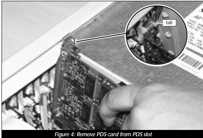
Figure 4: Remove PDS card from PDS slot
