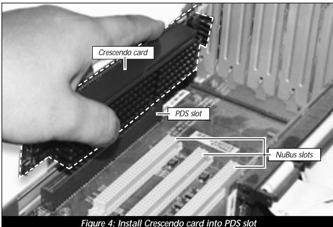
Figure 4: Install Crescendo card into PDS slot
