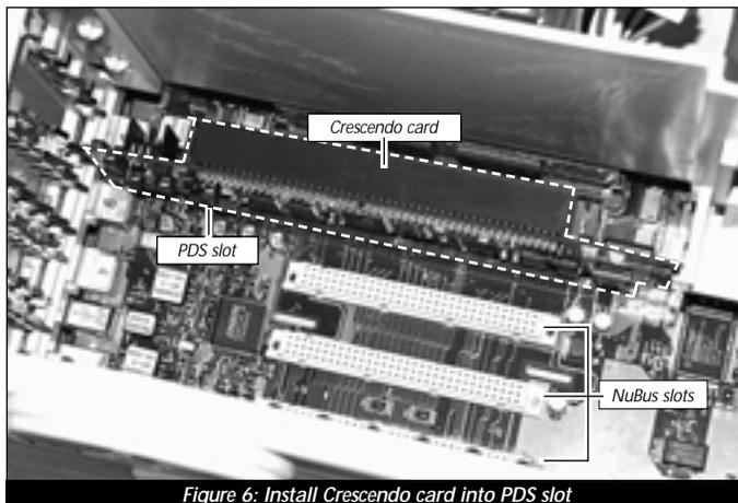
Figure 6: Install Crescendo card into PDS slot
