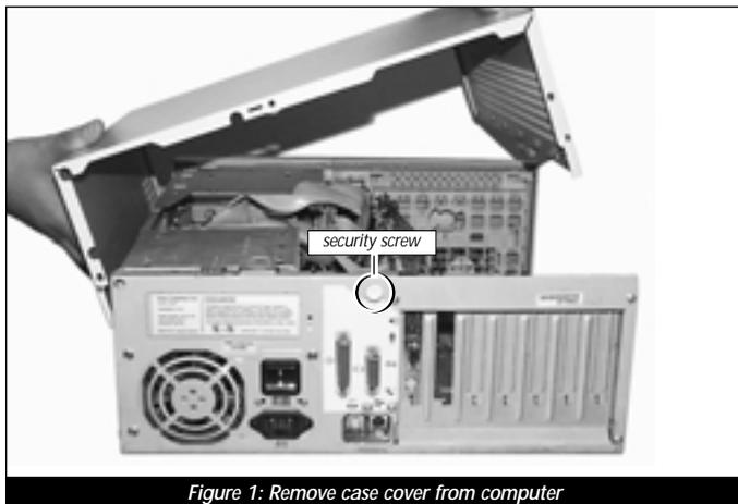
Figure 1: Remove case cover from computer
