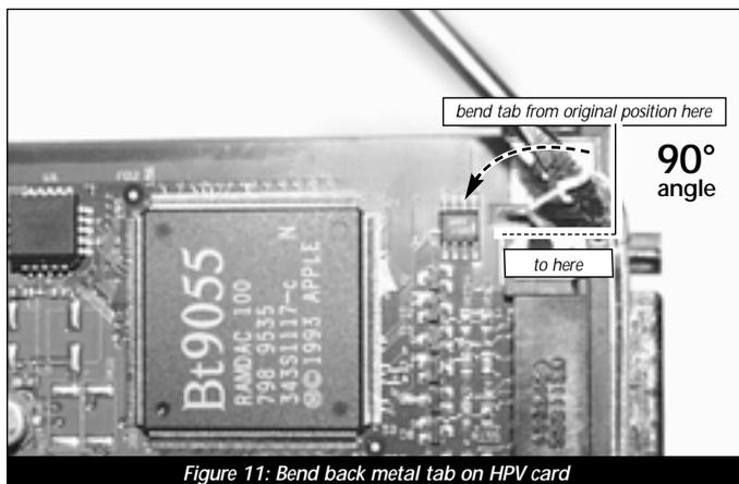
Figure 11: Bend back metal tab on HPV card
