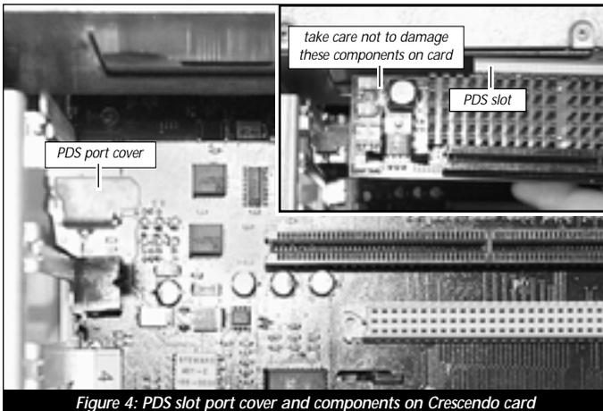
Figure 4: PDS slot port cover and components on Crescendo card
