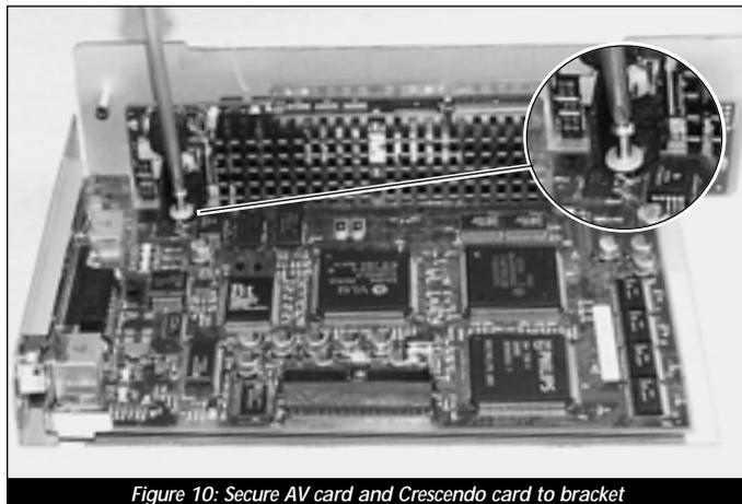
6. With the Crescendo and AV cards securely mounted onto the bracket, align the bracket over the PDS slot. Make certain the metal tab on the bracket slides into the inner slot on the side of the computer's case (**Figure 11**). Gently press down on the bracket so that the Crescendo plugs into the PDS slot.
