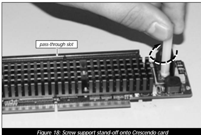
Figure 18: Screw support stand-off onto Crescendo card
