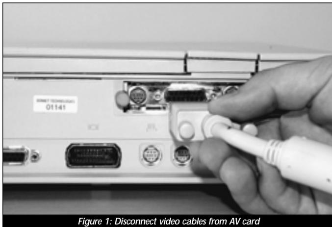
Figure 1: Disconnect video cables from AV card
