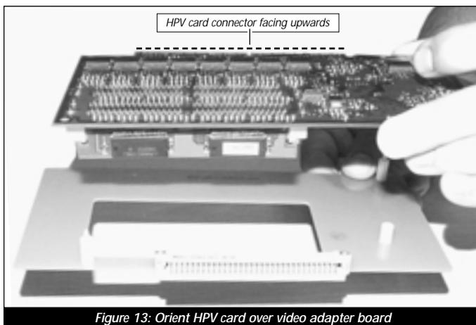
Figure 13: Orient HPV card over video adapter board
