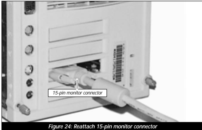
Figure 24: Reattach 15-pin monitor connector
