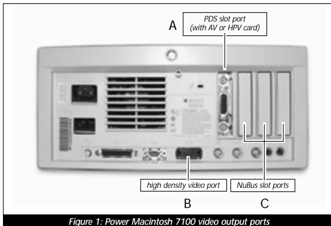
Figure 1: Power Macintosh 7100 video output ports
