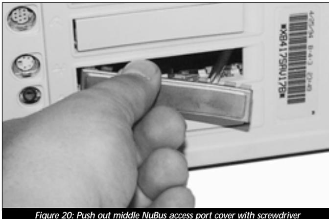
Figure 20: Push out middle NuBus access port cover with screwdriver
