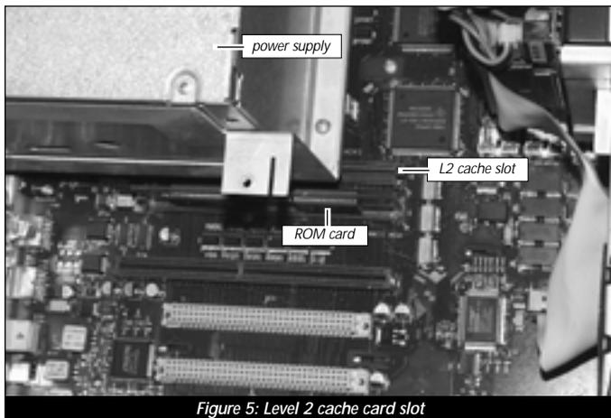
Figure 5: Level 2 cache card slot
