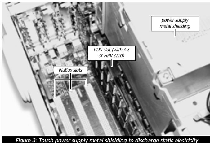
Figure 3: Touch power supply metal shielding to discharge static electricity
