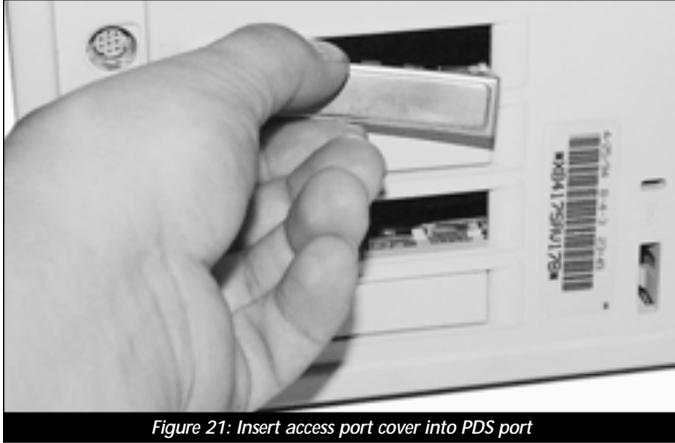
Figure 21: Insert access port cover into PDS port
