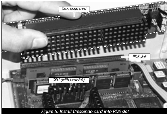
Figure 5: Install Crescendo card into PDS slot
