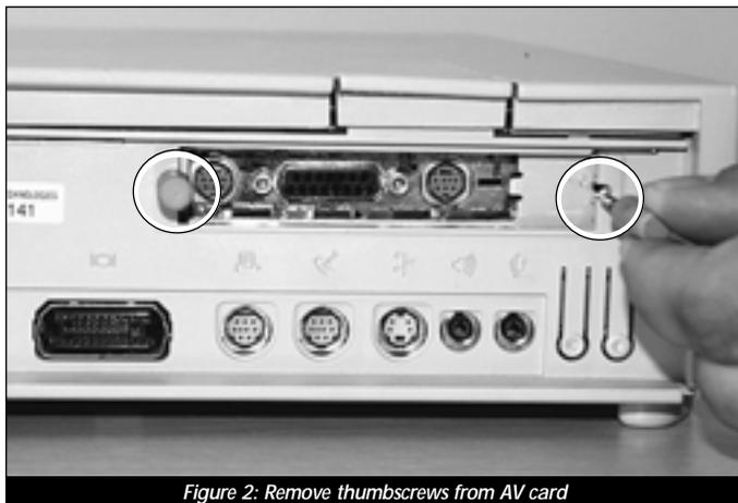
Figure 2: Remove thumbscrews from AV card
