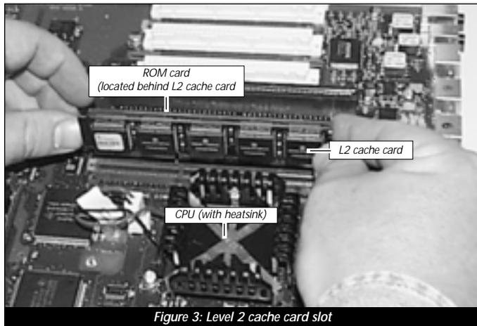
Figure 3: Level 2 cache card slot
