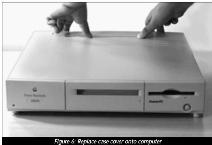
Figure 6: Replace case cover onto computer
