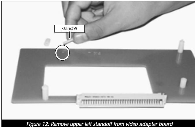
Figure 12: Remove upper left standoff from video adapter board
