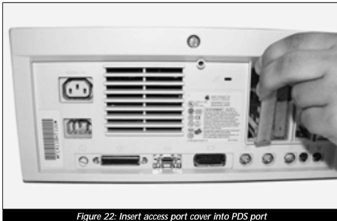
Figure 22: Insert access port cover into PDS port
