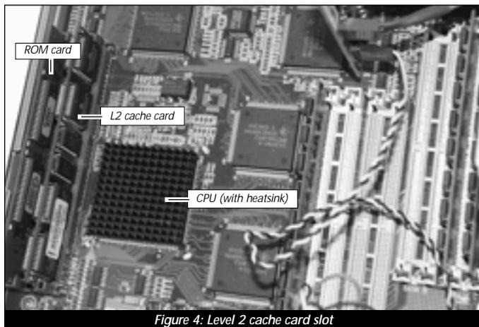
Figure 4: Level 2 cache card slot
