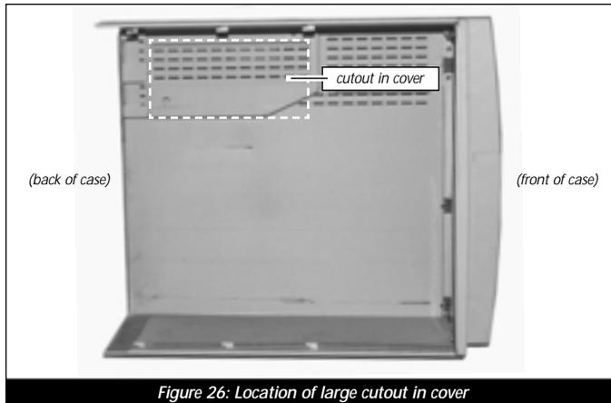
2. **Carefully** replace the cover onto your computer by slanting the front end of the cover over the computer (**Figure 27**). Confirm the inner grooves of the bottom of the case align with the tabs in the cover. As you slide back the cover, the top of the video adapter board and attached flex cable should fit nicely into the cutout of the cover. When the cutout of the cover clears the connector, you can lower the cover into place.
