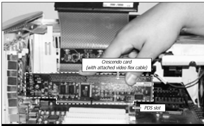
Figure 20: Install Crescendo card into PDS slot
