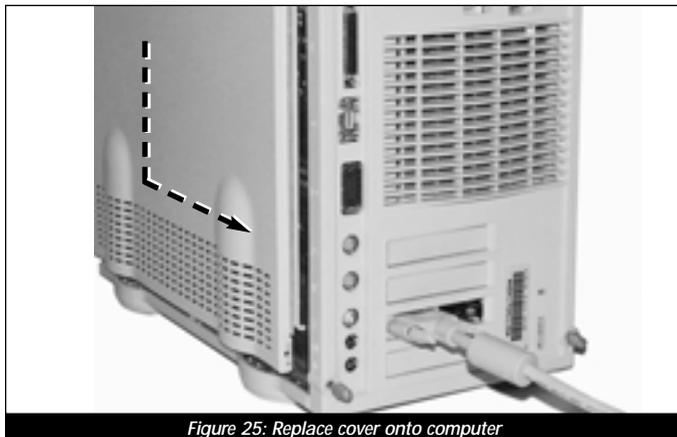
Figure 25: Replace cover onto computer
