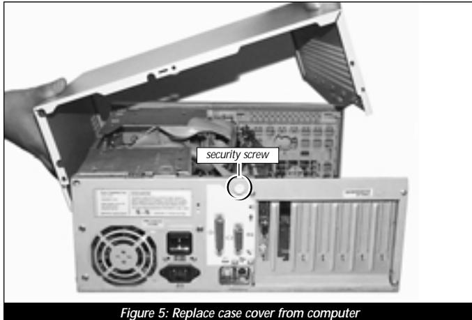
2. Return the computer to your computing area and reconnect the power and peripheral cables.
