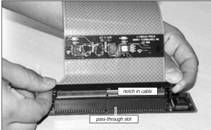
Figure 19: Attach video flex cable to Crescendo card
