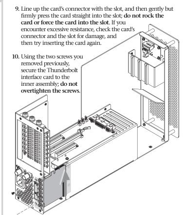
11. Grasping the outer case, gently push the inner assembly back inside.
