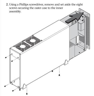
3. Grasping the outer case with one hand, push the inner assembly into the outer case, and then gently pull out the inner assembly. Set aside the outer case.
