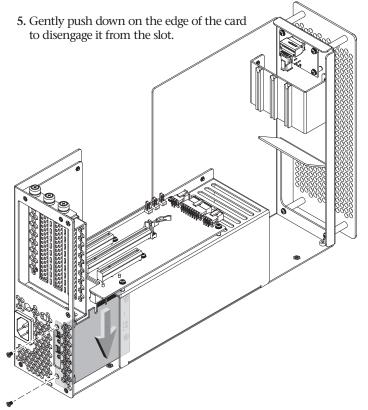
6. Grasping the card by its edges, rotate the bracket out of the inner assembly, and then pull out the card. Set aside the card on flat surface, component side down.
