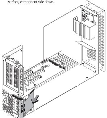
7. Remove the Thunderbolt 3 upgrade card from its packaging, handling the card by its bracket.
