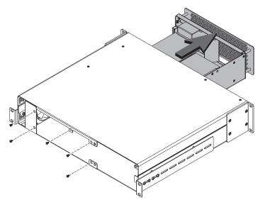
Push the inner assembly into the outer case, and then gently pull out the inner assembly. Set the inner assembly on a flat, level surface.
