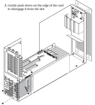
6. Grasping the card by its edges, rotate the bracket out of the inner assembly, and then pull out the card. Set aside the card on flat
