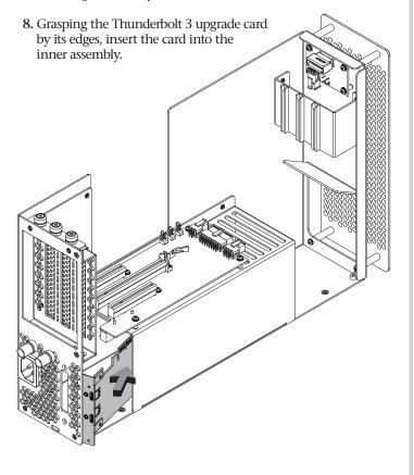
9. Line up the card's connector with the slot, and then gently but firmly press the card straight into the slot; do not rock the card or force the card into the slot. If you encounter excessive resistance, check the card's connector and the slot for damage, and then try inserting the card again.
