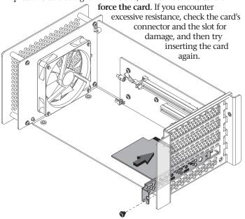
**8.** Secure the Thunderbolt 3 upgrade card using the screw you removed previously; **do not overtighten the screw**.
