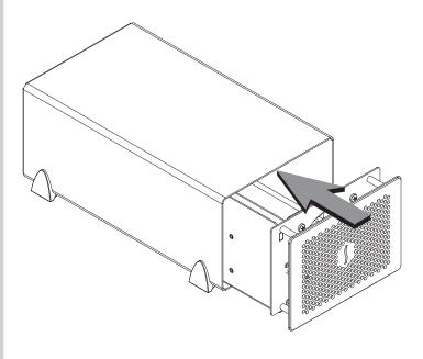
10. Turn the assembled Echo chassis upside-down, and then using the four screws you removed previously, secure the outer case to
