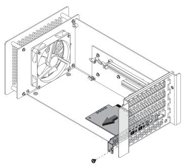
5. Grasping the Thunderbolt interface card by its edges, gently disengage the card from its slot, and then remove the card from the chassis. Set aside the card on flat surface, component side down
