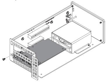
12. Place your hand on top of the outer case, and then gently push the inner assembly back into the outer case.
