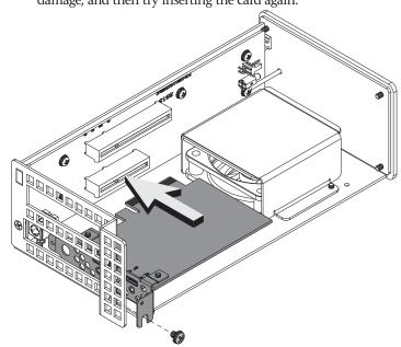
Secure the top of the Thunderbolt 3 interface card mounting bracket using the screw you removed previously; do not overtighten the screw.
