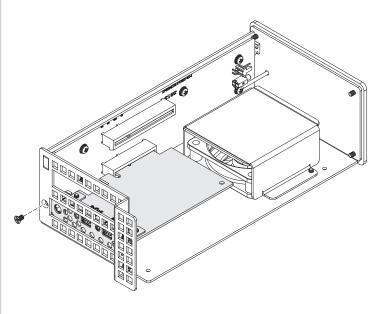
**5.** Remove and set aside the screw securing the top of the Thunderbolt 2 interface card mounting bracket.
