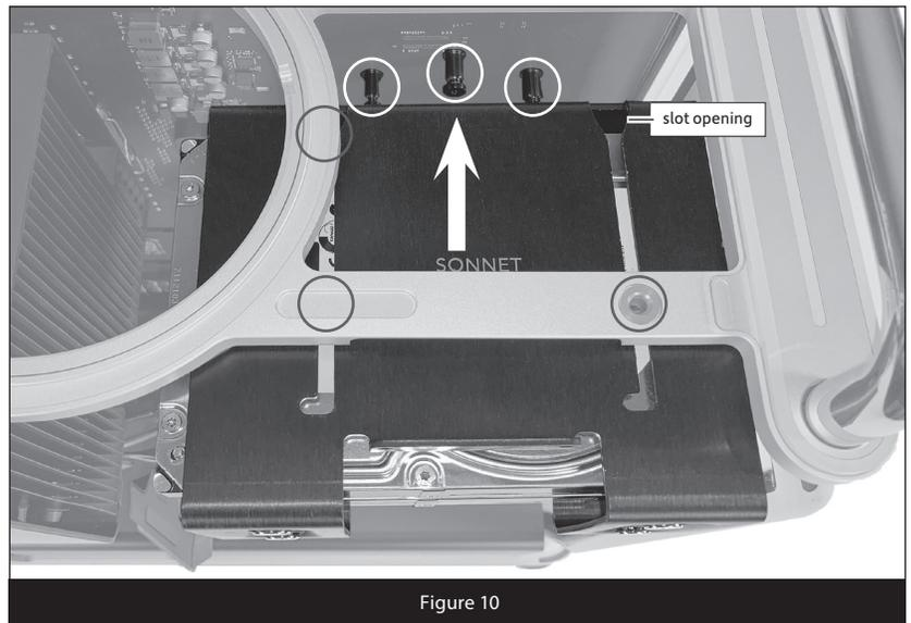
6. With the Fusion Flex J3i primary bracket's top tab against the computer's frame, slide the bracket to the right until it stops; the tab should be centered between the two screw holes in the frame (Figure 11).
