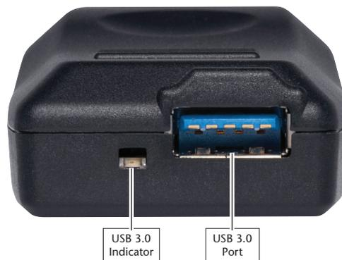
**USB 3.0 Port** – Connect either the included USB 3.0 cable or another USB 3.0 cable between the adapter and your computer.
