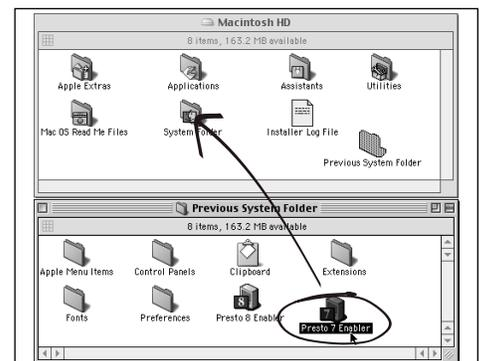
Figure 13: Copy Presto 7 Enabler to System Folder
