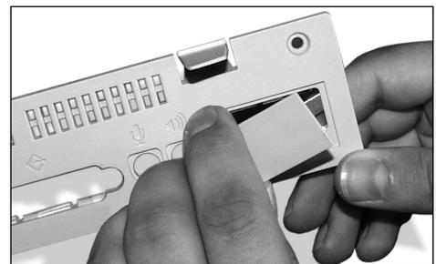
Figure 3: Remove PDS access port cover
