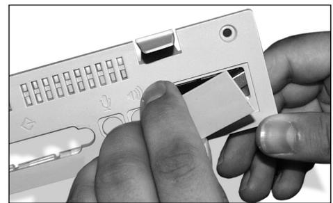
Figure 3: Remove PDS access port cover
