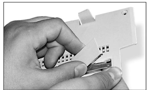
Figure 3: Remove PDS access port cover
