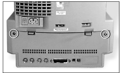
Figure 1: Remove security screws
