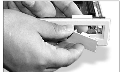
Figure 2: Remove PDS access port cover
