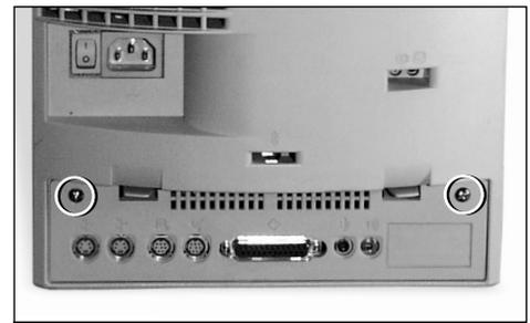
Figure 1: Remove security screws
