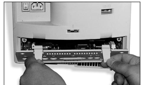
Figure 2: Unlatch and remove back panel
