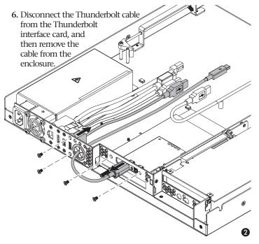
7. Grasping the Thunderbolt interface card by its edges, pull out the card from its slot. Set aside the card on flat surface, component side down.
