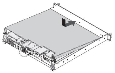
**16.** Insert the top cover under the top edge of the enclosure, lower the lid, and then secure it with the captive thumbscrews; your upgrade is complete.
